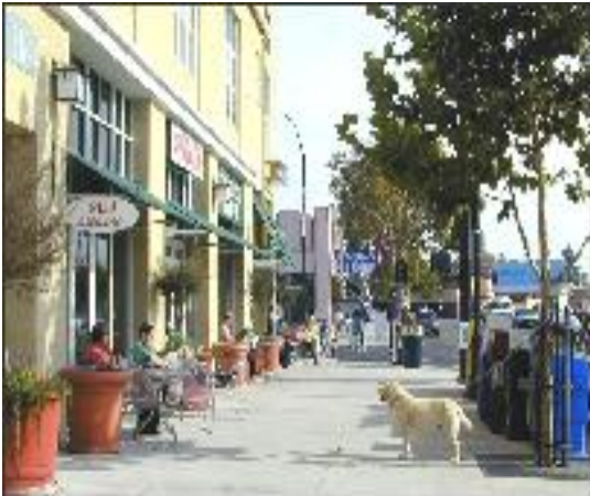
Figure 7.6. An example of a wide urban sidewalk showing all three zones, with café tables in the transition zone.
