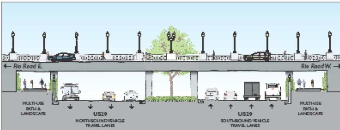
**Figure 7.17. This cross section of the recommended grade-separated intersection at US 29 and Rio Road shows the travel lanes, median, and pedestrian/bicycle facilities as they go under the overpass. Similar conditions are expected at the other grade-separated intersections along US 29.**
