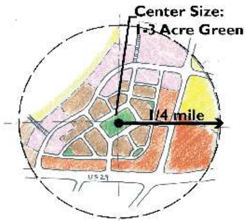
Figure 5.7. Concept Diagram of a Mixed Use Neighborhood Shown with a central public open space
