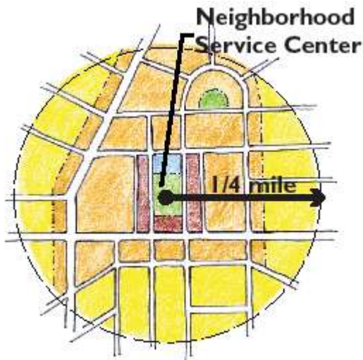
Figure 5.2. Concept Diagram of a Residential Neighborhood Shown with a Neighborhood Service Center
